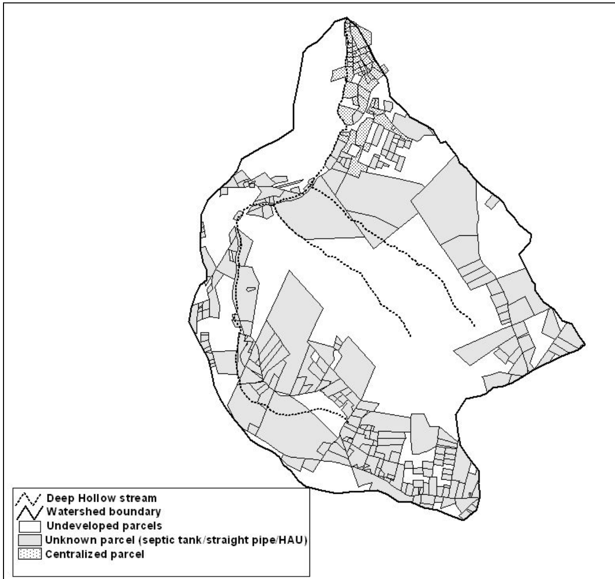
Figure 22: Parcel based inventory of wastewater treatment systems in the Deep Hollow watershed
